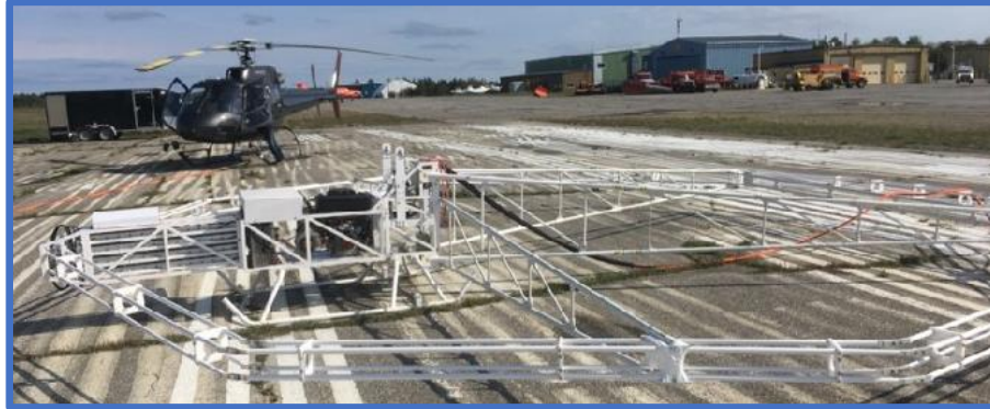
Image of Loop Transmitter System with Helicopter. Features on-board power generation and ease-of-flight for low noise and high signal quality
